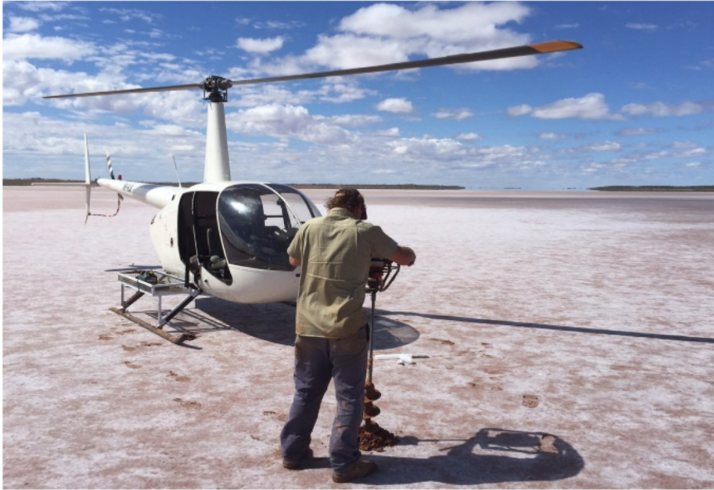
Figure 8: Hand held auger drilling
